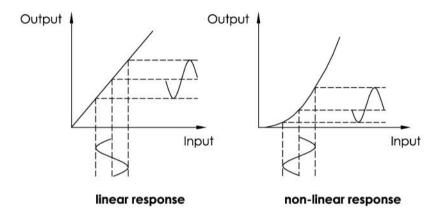
Because the non-linearity have a imperfect diode response, the waveform of output is obviously distorted, whereas the one of linearity is proportional to input. When the distorted signal is converted to frequency domain, it consists of the desired fundamental carriers and a series of related harmonics named intermodulation products. The products are mathematically related to the original frequencies:
